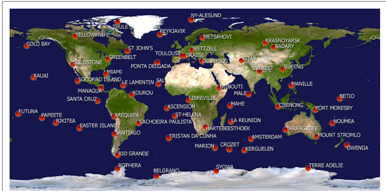
Figure 3.3: Map of Doppler Orbitography and Radiopositioning Integrated by Satellite (DORIS) ground network. The coverage is very well distributed in both hemispheres; the only area with sub-par coverage is the North Pacific. This image is from the International Doris Service (IDS) website: http://ids-doris.org/ .
